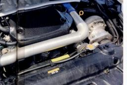
Let's get one thing straight: Nissan hasn't simply bolted on a supercharger, whacked the boost up and gained lashings of extra power nice and easily. Instead, the unit is a clutch-operated centrifugal blower with a front-moun intercooler designed for reliability. This is controlled by a button next to the gear lever which simply savs 'Novidem - Kompressor': Novidem (based in Switzerland) being the company that was tasked with building the supercharger.
