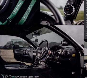
INTERIOR: Recaro Polo Position fixed-back bucket seats, stripped rear, all S15 equipment adjusted to correctly deliver 1JZ engine readings, Takata DRIFT III harnesses, Nardi perforated leather steering wheel, Defi gauges
