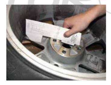
3. Lay the template resulted inside the wheel.
