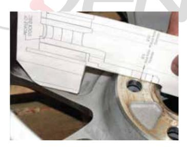
4. Verify that the edge of the caliper does not touch the rim or any of the spokes. We recommend a minimum of 2mm clearance.
